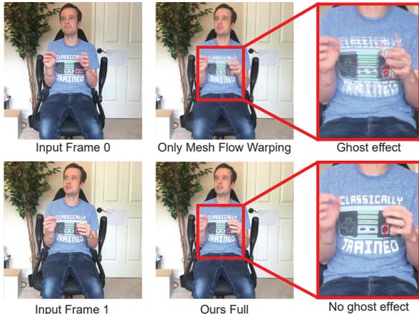
Figure 5. A ghost effect example. **Left:** two input frames. **Top-right:** ghost effect from using mesh flow only. **Bottom-right:** sharp features with further warping by optical flow.
