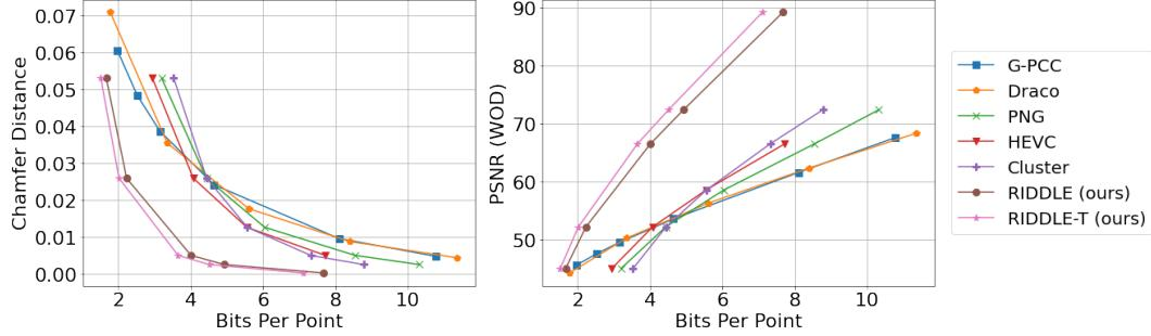
Figure 4. **Evaluation of the compression methods with geometric metrics on the Waymo Open Dataset val set.** *Left:* Chamfer distance v.s. bit per point (bpp); *Right:* PSNR v.s. bpp. At a certain bitrate, lower the Chamfer distance or higher the PSNR, better the reconstruction quality.
