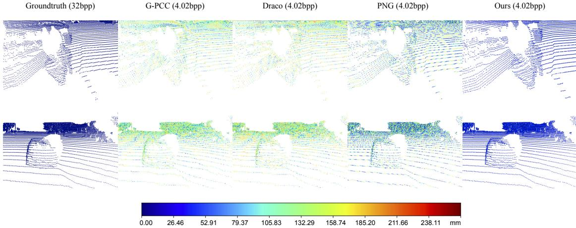
Figure 7. **Visualization of reconstructed point clouds, colored by per point Chamfer distance** (error bar colormap on the bottom). From left to right: raw, G-PCC, Draco, PNG and RIDDLE (ours). It is clear that our method, under the same bit per point, has much less distortion. Best viewed in color with zoom in.
