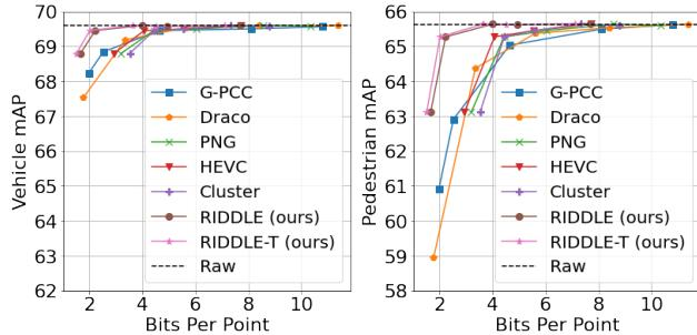
Figure 6. **Impact of lidar data compression to 3D object detection quality on the Waymo Open Dataset val set.** We train PointPillars [17] detectors using the raw point clouds (with no compression) from the WOD train set and evaluate them with the compressed point clouds (or point clouds from the compressed range images) on the WOD validation set.
