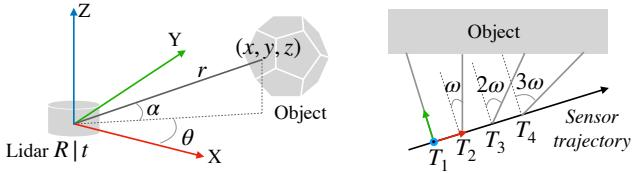
Figure 1. **Illustration of laser shots.** *Left:* A single laser shot. *Right:* Laser shots across time (in a bird’s eye view). We show four consecutive laser shots (with delta azimuth angle  $\omega$ ) that measure the ranges from the (moving) sensor to the object. To convert the range values to a point cloud, we need to know the ranges, the shot angles, as well as the sensor poses at each shot.
