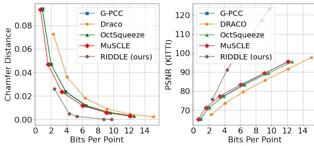
Figure 5. **Evaluation of the compression methods with geometric metrics on the SemanticKITTI test set.** We only present our intra-frame model here as the per pixel sensor pose is unavailable in SemanticKITTI.
