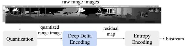
Figure 2. **The deep delta encoding pipeline for lidar range image compression.** Given a lidar range image, we first quantize the attribute values and then run inference of the predictive model on the quantized range image to derive residuals. Finally we use entropy encoders to compress the residuals to a bitstream.
