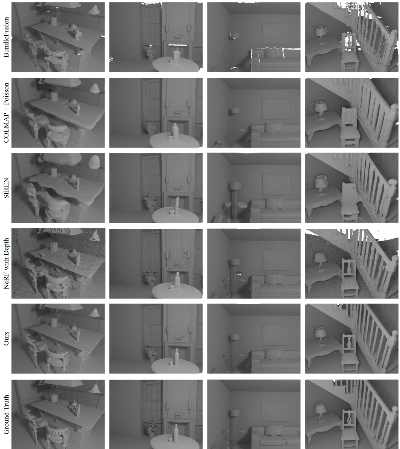
Figure 9. We show a qualitative comparison of synthetic scene reconstructions obtained using our method and several baseline methods. The BundleFusion reconstruction is incomplete in some regions, screened Poisson and SIREN attempt to fit noise in the depth data, while the NeRF reconstruction suffers from noise in the density field. Our method manages to fill in gaps in geometry, while maintaining the smoothness of classic fusion approaches.
