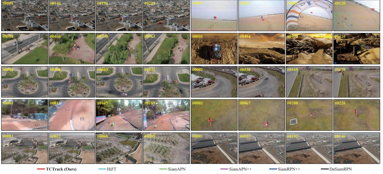
Figure 1. Qualitative comparisons among TCTTrack and other state-of-the-art trackers. Missing trackers are denoted as "x" using the corresponding color. It clearly shows that our tracker achieves superior performance in various challenging aerial scenarios, especially in fast motion, low resolution, severe occlusion, and camera motion. Best viewed on the screen with high-resolution.
