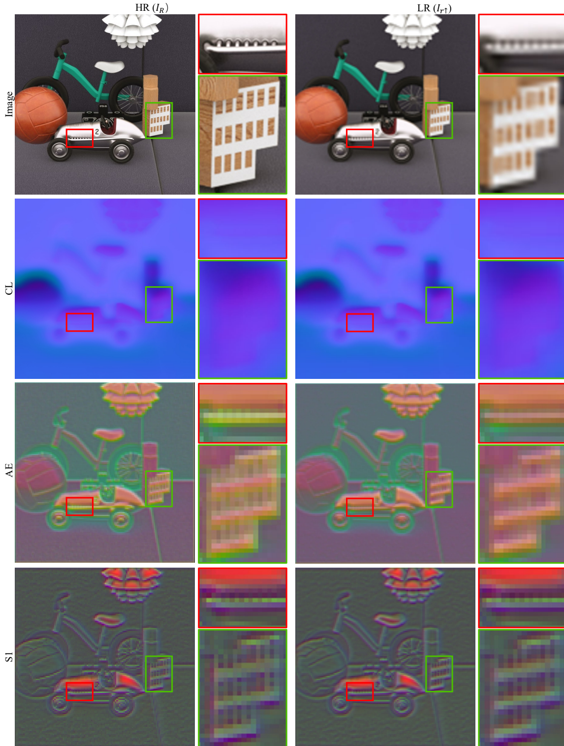
Figure 2. The HR and LR feature maps (2nd to 4th row) generated from the HR and LR right view images (1st row) by different feature-learning methods. Feature maps are visualized by projecting the high-dimensional feature spaces onto a three-dimensional space ( i.e. , RGB) using PCA. Note that, due to dimension reduction, the original feature spaces may contain more information than displayed here. This scene is from the Inria_SLFD dataset and simulated with an asymmetric factor of 4 and under the BIC degradation.
