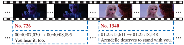
Figure 5. Examples of how to cut a movie into a series of video clips according to subtitle files. Note that the subtitle files contain both starting and ending time-stamps for each video clip.
