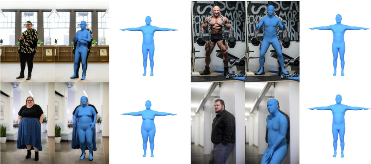
Figure R.8. Failure cases. In the first example (upper left) the weight is underestimated. Other failure cases of SHAPY are muscular bodies (upper right) and body shapes with high BMI (second row).
