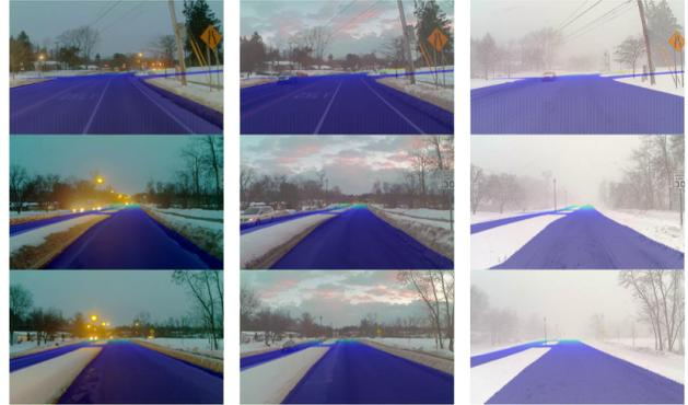
[Figure 11](#). Generated ground truth depth masks for each pixel lying in the road area. Lighter blue indicates farther depth.
