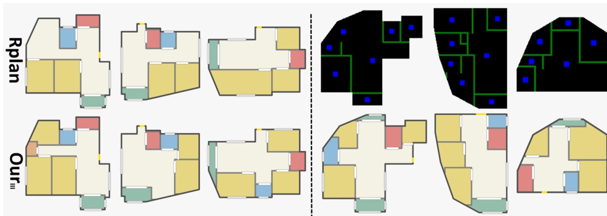
Figure 3. Layouts with non-axis aligned edges. Left: successful examples. Right: Rplan fails but our model succeeds.
