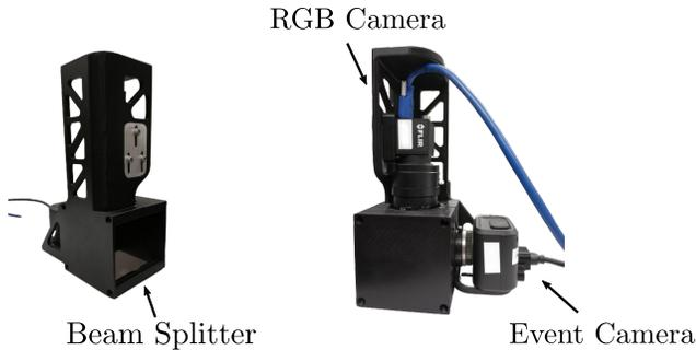
Figure 6. Beam-splitter with an event and a standard camera.
