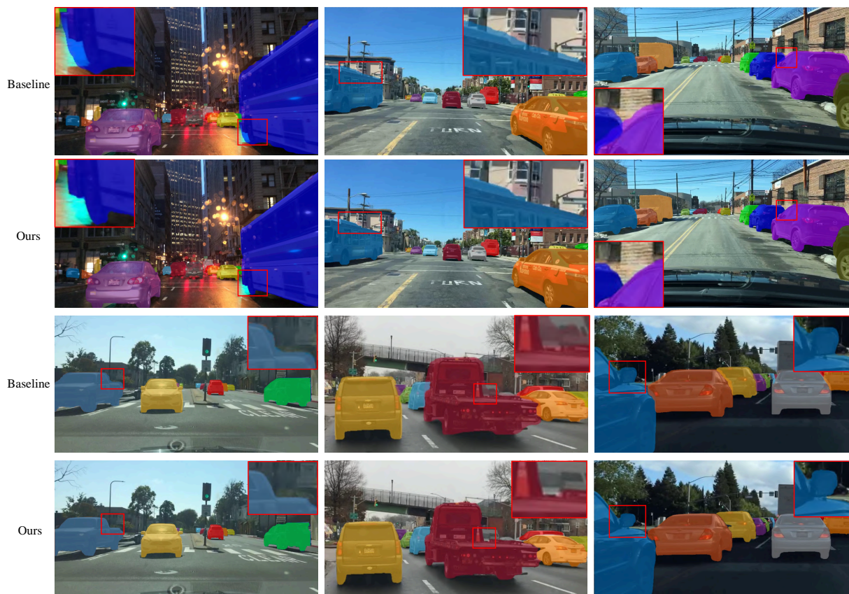
Figure 3. Qualitative comparisons with baseline method Mask R-CNN [7] and our Mask Transfimer on BDD100K [15] val set. Mask Transfimer produces more correct and natural segmentation results by revealing details for high-frequency regions.
