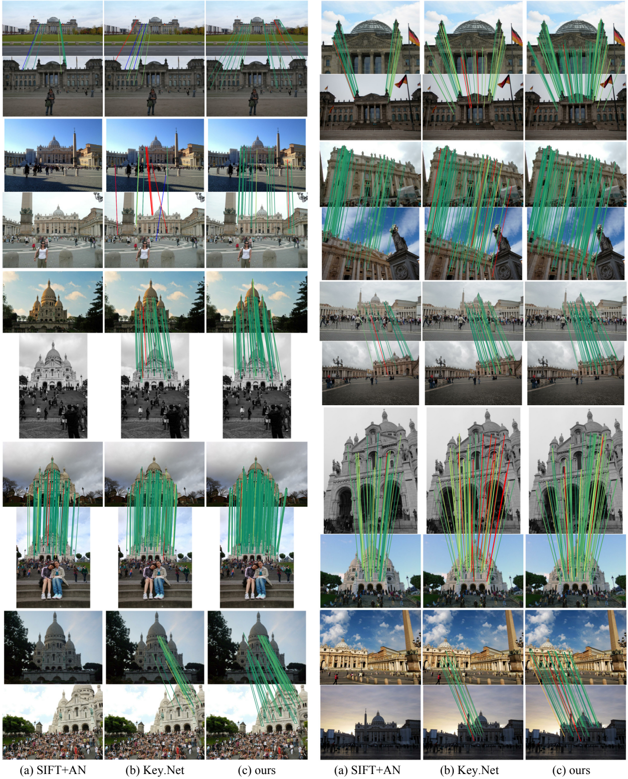
Figure 5. Visualization of the predicted matches in IMC2021 [7], with HardNet descriptor [10], DEGENSAC [4] with AdaLAM [3]. Matches above the 5-pixel error threshold are displayed in red, and matches below are color-coded according to errors between 0 (green) to 5 pixels (yellow). Matches without a depth estimate are displayed in blue. We use 1,024 keypoints to compare with SIFT+AN [9, 11], Key.Net [2], and ours.
