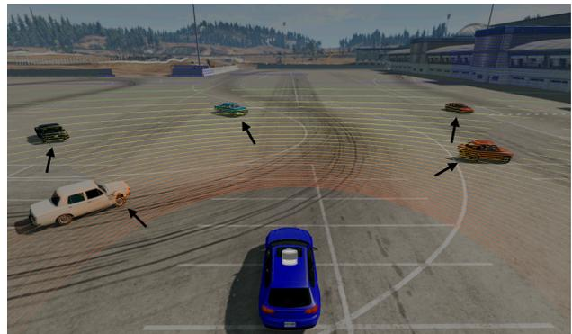
Figure 6. LiDAR scene setup of CrashD. For each car, a black arrow indicates its damaged area, which is ensured to be visible from the sensor viewpoint. Image used with courtesy of BeamNG GmbH.
