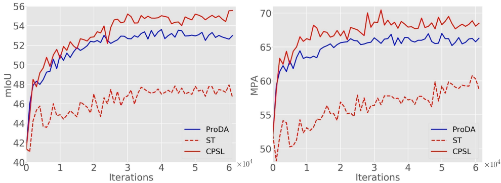
Figure 1. The mIoU (left) and MPA (right) scores evaluated on the validation set during the training.
