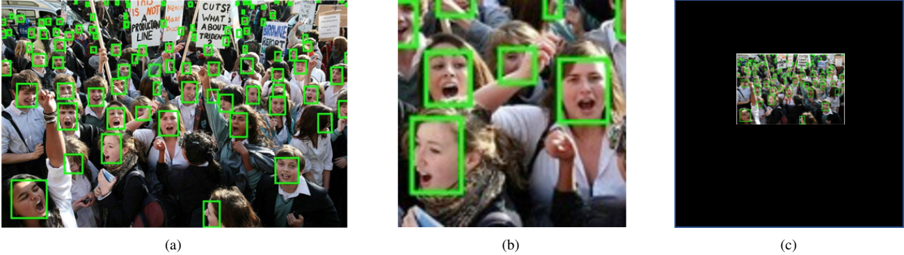
Figure 1: An image is augmented by multi-scale training and data-anchor-sampling respectively. (a) An original image. (b) The image in (a) is augmented by the random crop strategy. The native image information is less than the original image. Note that this image may blur the image when the expand ratio is large. (c) The image in (a) is augmented by the data-anchor-sampling strategy. This brings a large amount of padding area, that reduces the learning difficulty of the detector on negative anchors. Thus, the fore-ground information in native image information is reduced remarkably.
