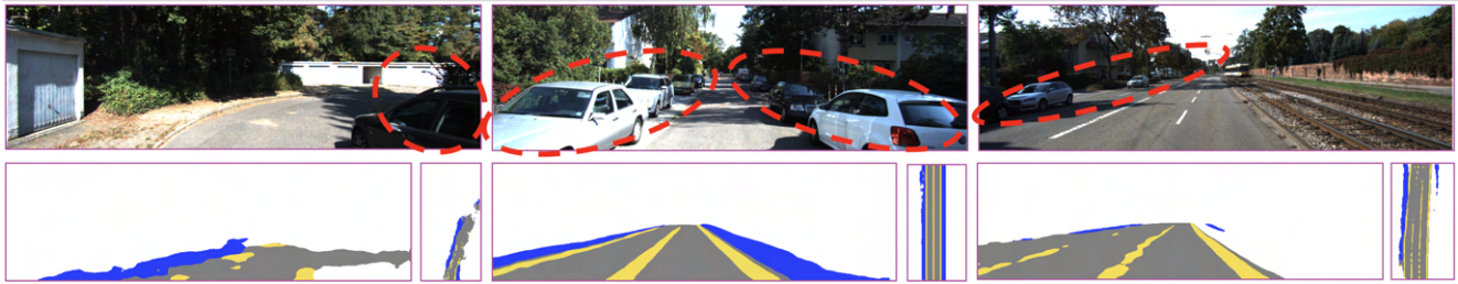
Figure 6. First row: RGB. Second row: predicted OSP and HST. We can see that our model is able to handle various occlusions, e.g. occluded curved road or road occluded by cars, very in both perspective and top view.
