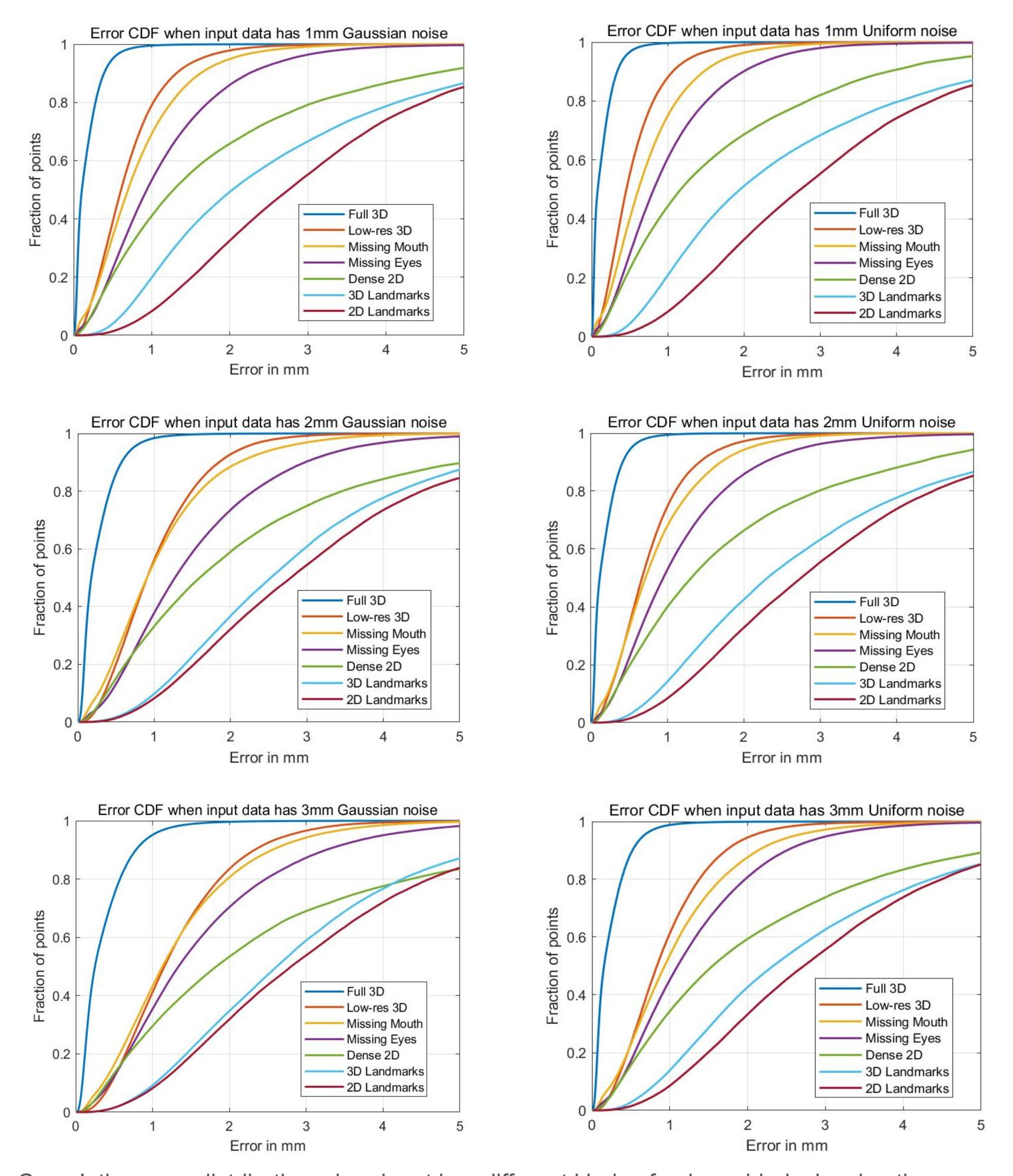
Cumulative error distribution when input has different kinds of noise added, showing the fraction of reconstructed vertices with less than a given threshold error. The overall relationship between data types is the same as in the no noise analysis.
