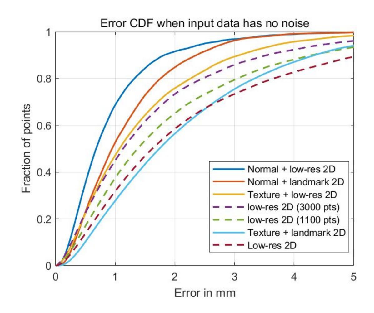
Cumulative error distribution, showing the fraction of reconstructed vertices with error less than a given threshold. This plot contain extra input data types not shown in Figure 2. Note that the 'low-res 2D' data type has 800 2D points, while 'low-res 2D (1100 pts)' and 'low-res 2D (3000 pts)' have correspondingly 1100 and 3000 points. These are similar to 'Dense2D', just with many fewer points, analogous to the LowRes3D datatype's reduction from Full3D.
