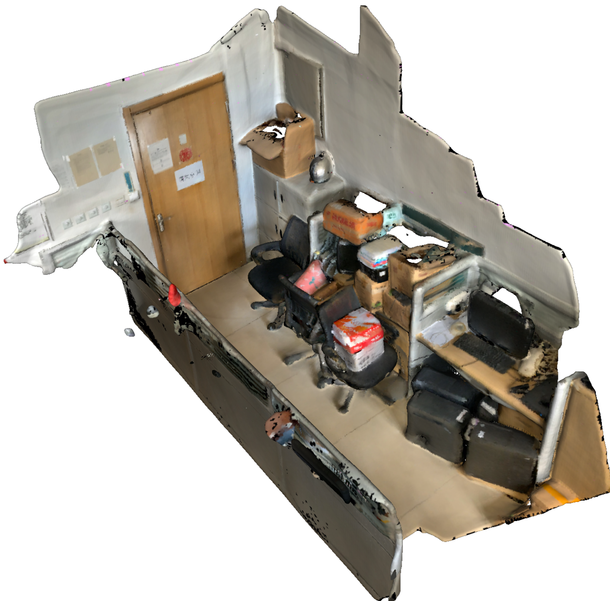
Figure 8. Surface reconstruction of a real scanned scene with texture.
