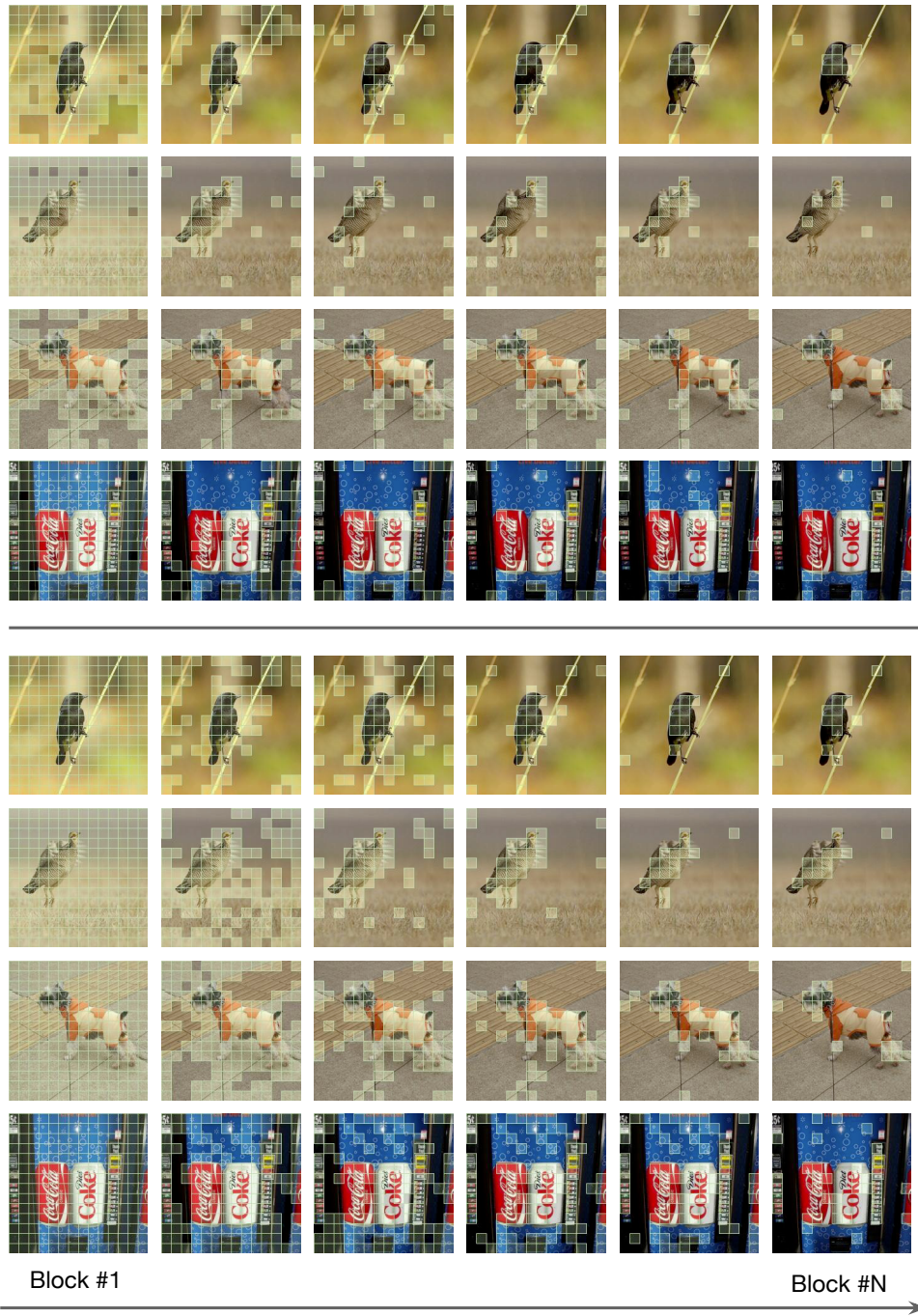
Figure 3. Visualization of selected patches at different blocks with T2T-ViT [2] (Above) or DeiT [1] (Below) as the vision transformer backbone respectively. Green color denotes the patch is kept.
