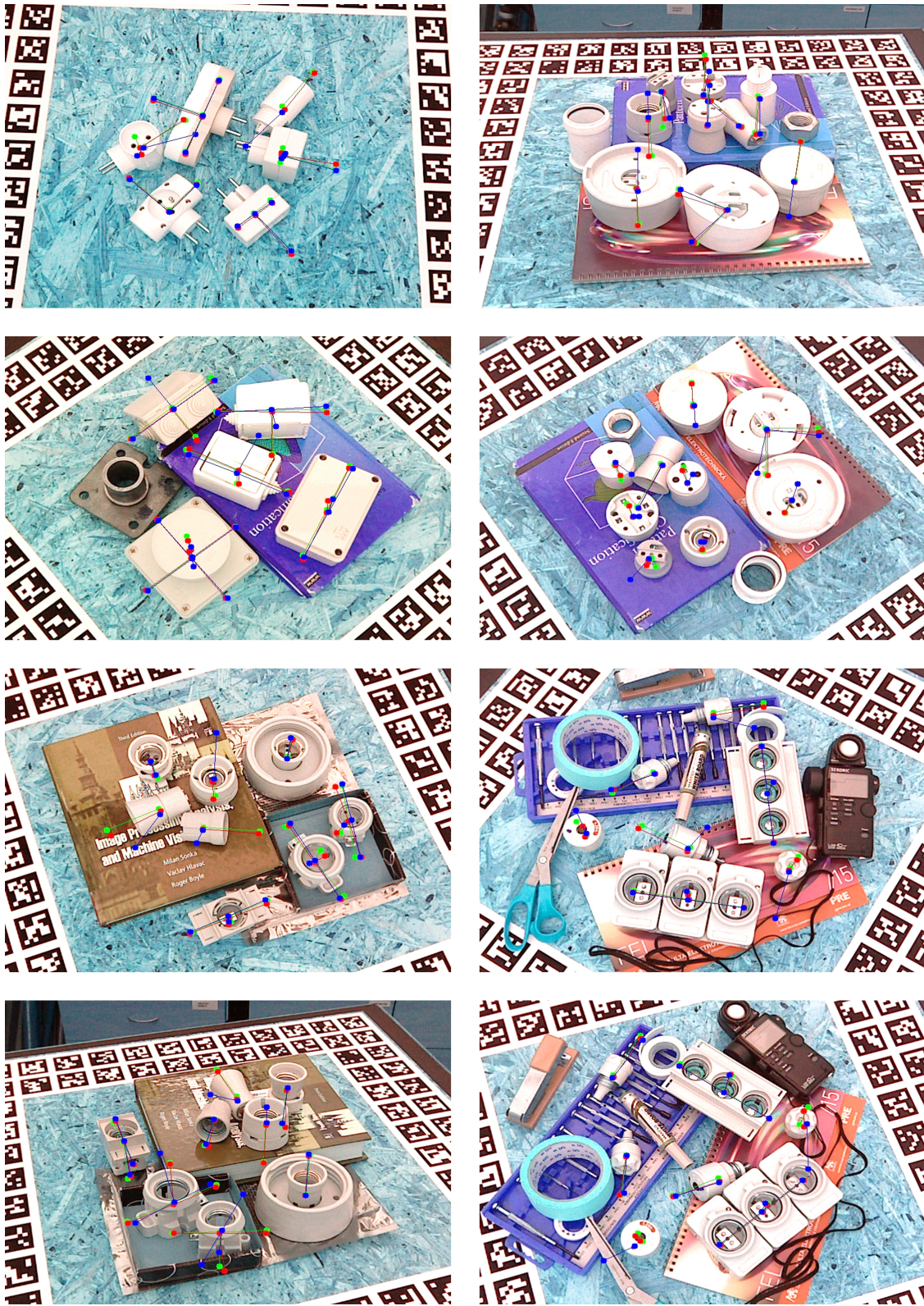
Figure 8. Visualization on the T-LESS dataset with different training loss. The green, red, and blue lines represent the ground truth pose, the result from A(M)GPD loss, and the result from ADD(S) loss, respectively.
