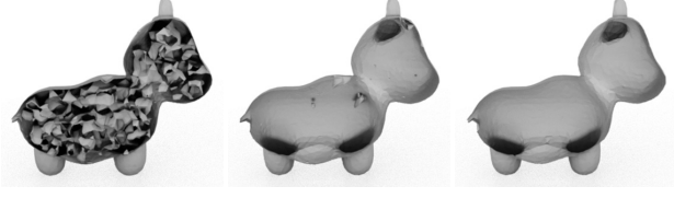
Figure 17. Cross sections of shapes optimized without regularization loss on SDF (left), with smoothness loss used by Liao et al. [11] (middle) and with our regularization loss (right). The random faces inside the object are removed by the regularization loss on SDF.
