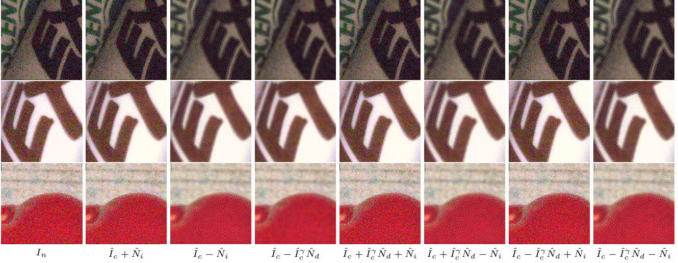
Figure S3. Generated synthetic noisy images by our proposed self-supervised augmentation strategy on the SIDD validation dataset.
