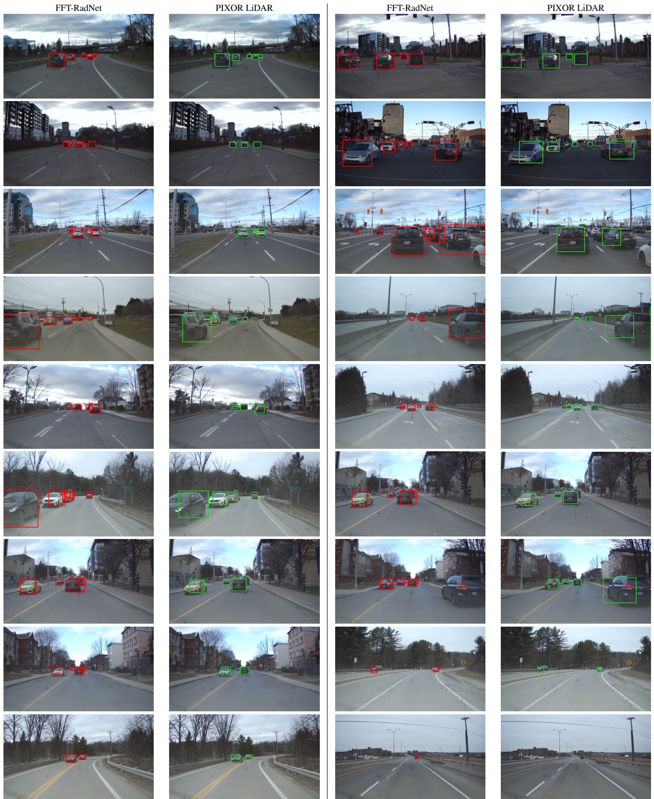
Figure 3. Examples of vehicle detection in complex scenes using either HD radar or LiDAR. Comparison between Pixor trained with LiDAR point clouds (‘PIXOR LiDAR’ columns, green boxes) and our proposed FFT-RadNet requiring only range-Doppler as input (‘FFT-RadNet’, red boxes). Note that radar detections are not limited to the first row of vehicles but can see up to the second one. Also, FFT-RadNet provides vehicles’ relative speed through Doppler measurements.
