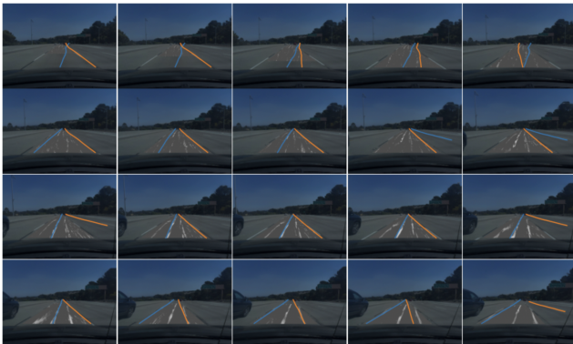
Figure 7. The first 20 frames (from left-top to right-bottom) of an attack scenario on LaneATT . The vehicle is deviating to right due to the attack.
