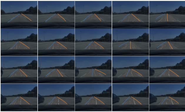
Figure 6. The first 20 frames (from left-top to right-bottom) of an attack scenario on PolyLaneNet . The vehicle is deviating to right due to the attack.
