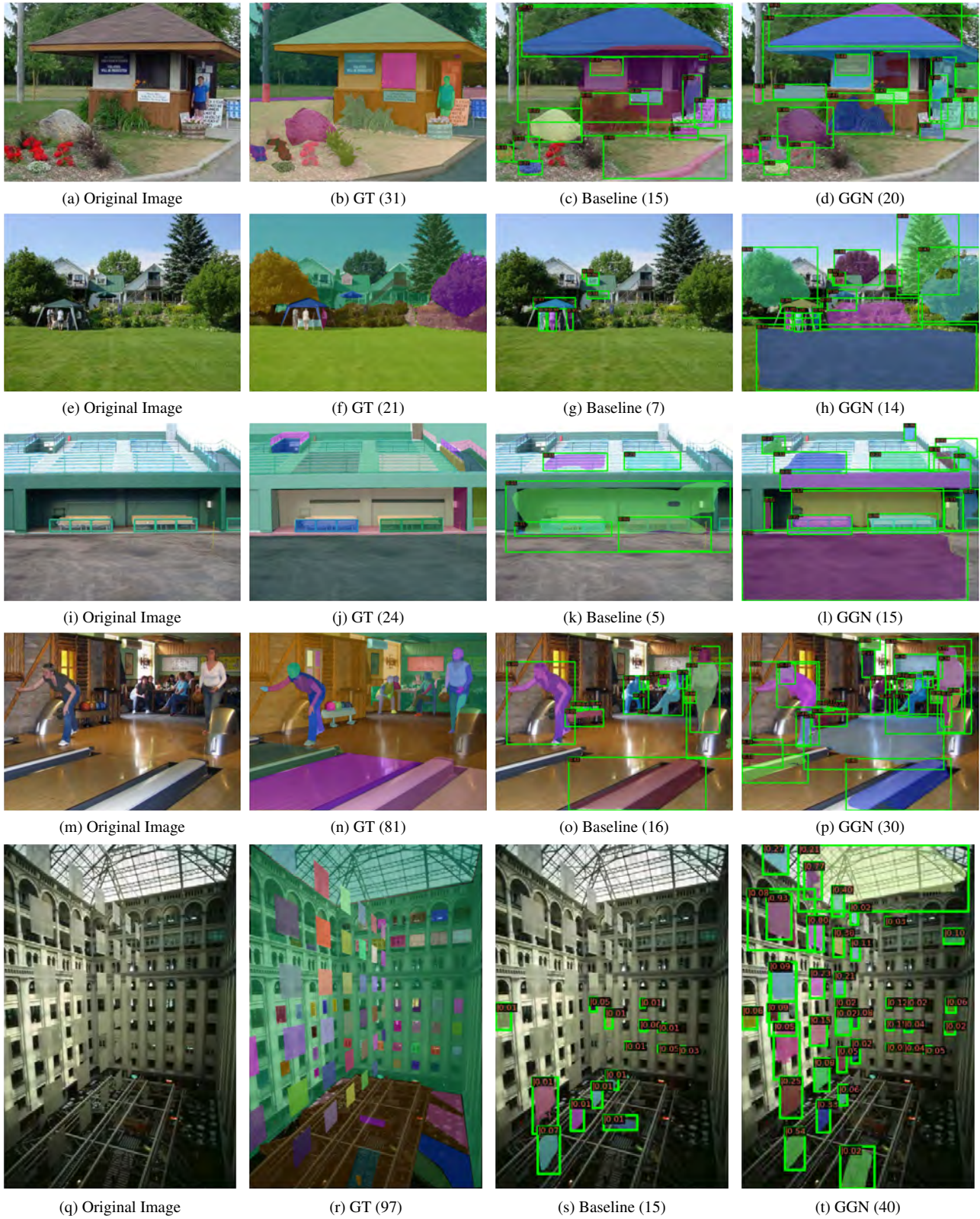
Figure 2. Visualization of GGN compared to baseline on ADE20k. We take top-100 scoring predictions for each of the methods. GGN detects significantly more true positive segments compared to baseline, including novel objects and stuff. Number in bracket represents number of retrieved segments.
