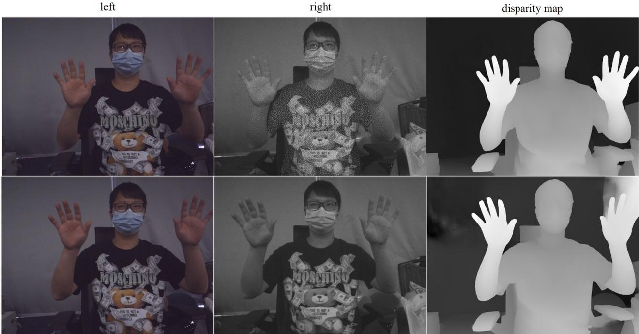
Figure 3. Qualitative comparison of our fusion method and the passive stereo method. The first column shows the left images, the second column shows the right images, and the last column shows the disparity maps. The first row shows the results of our fusion method (RAFT-OM-G is used), and the second row shows the results of the passive stereo method (RAFT-O is used).
