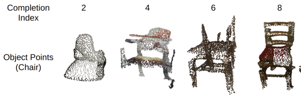
Figure 1. Point clouds of chairs with different partial indexes in ScanNet dataset. We see that small partial indexes refer to objects are occluded and partial, while objects with large partial indexes are more complete.
