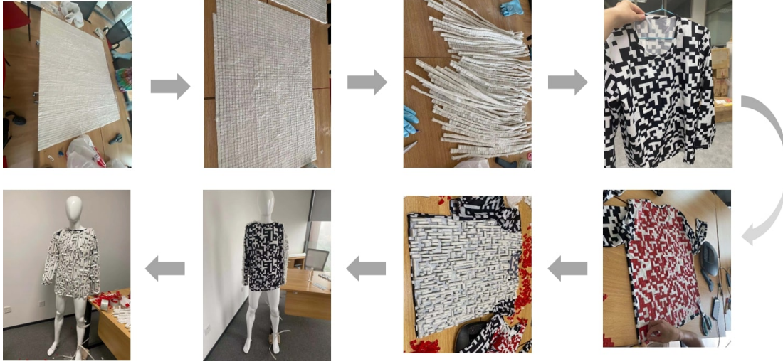
Figure S3. The manufacturing process of the “QR code” clothing. See Supplementary Video 2 for more details.
