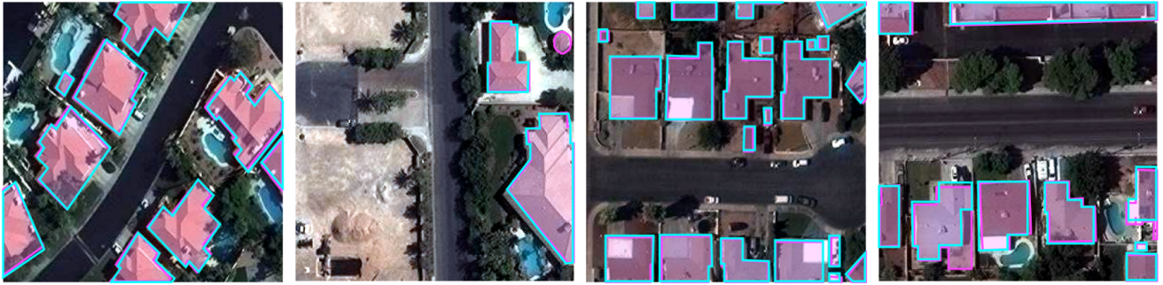
(a) Magenta: Ground truth polygons. Cyan: Results of the full PolyWorld method.
