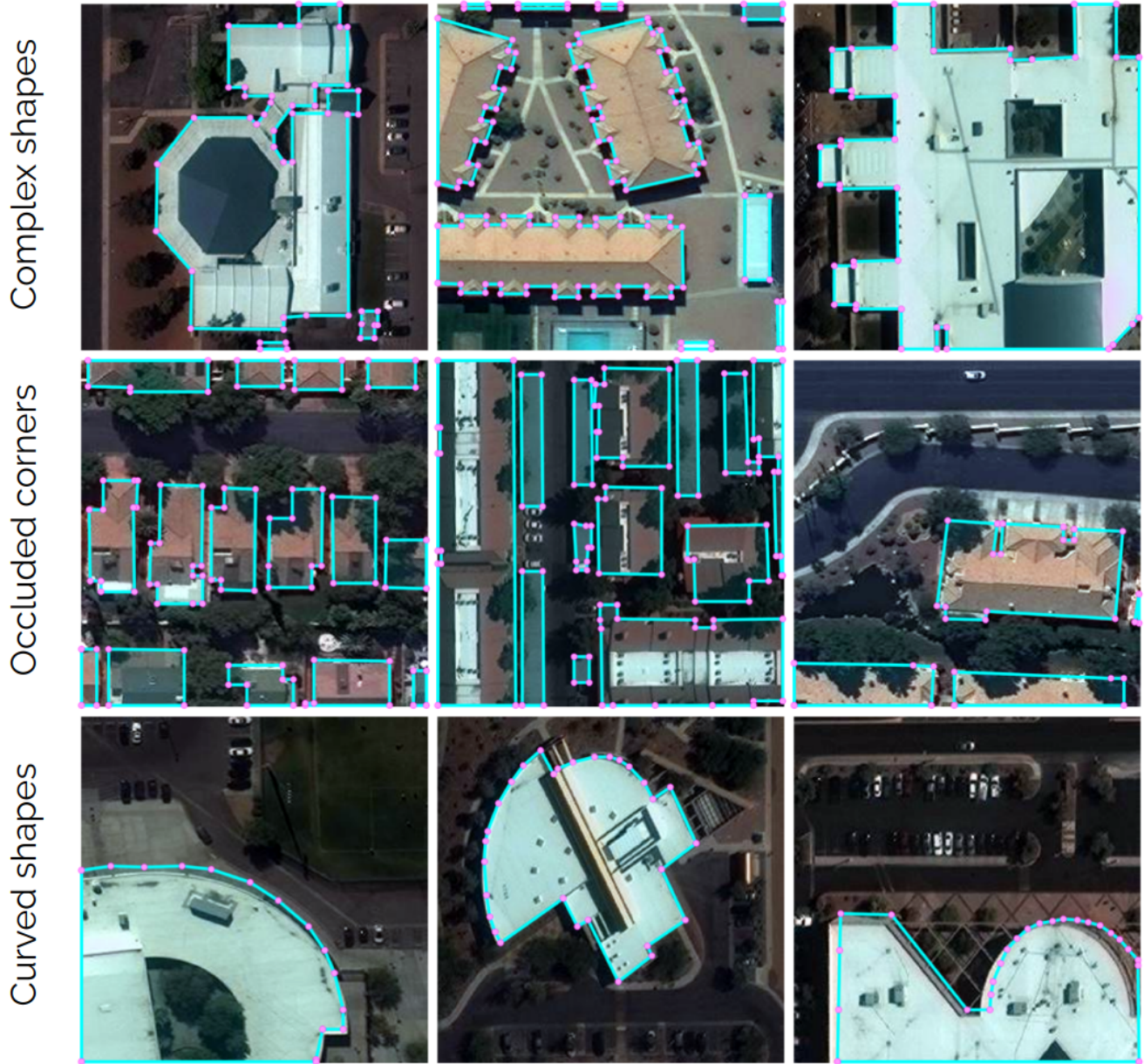
Figure 5. Results of PolyWorld on challenging images from the CrowdAI test dataset. First row: unusual and complex buildings. Second row: buildings with corners occluded by vegetation. Third row: buildings with curved walls.
