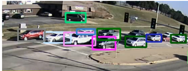
Figure 1. Challenges of tracking vehicles within a camera view – Tracking vehicles in real-world scenarios is challenging due to heavy occlusions, e.g., when vehicles wait at a traffic light. Some vehicles are not detected while they are occluded which often leads to track fragmentation or identity switches.
