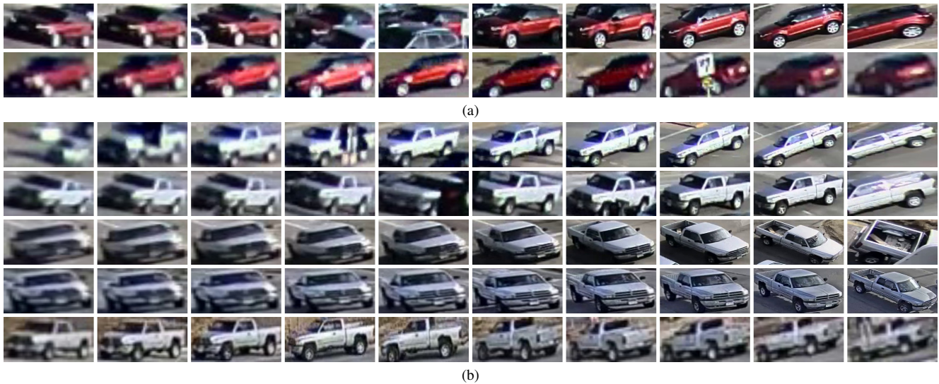
Figure 5. Qualitative Multi-camera Tracking Results – Each row shows a single-camera tracklet from a different camera. The upper track shows the effectiveness of our TRM. The lower track shows that with our approach, even with variation in viewing angles and lighting conditions, vehicles can be tracked through multiple cameras.
