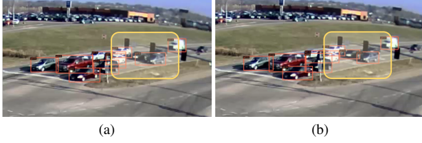
Figure 3. Examples of detected small and occluded vehicles. The left image shows the vehicle lost if without large input size and image patches strategies. The right image demonstrate our detection model can detect the small and occluded vehicles.
