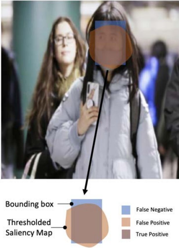
Figure 7. Definition of false negative, false positive and true positive using YOLOv5s.
