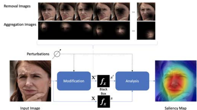
Figure 1. Diagram of our method MinPlus. The key idea is to analyze how the score varies when add or remove a part of the original image. The input-output function of the black-box is f_x . In this example, the saliency map corresponds to the most important parts used by a face verification algorithm.
