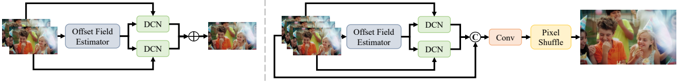
Figure 3. Framework of Video Frame Interpolation (VFI) sub-module (left) and Video Super-Resolution (VSR) sub-module (right).
