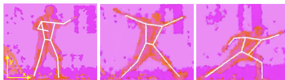
Figure 2. Skeleton data overlayed on depth data from FFD. Only 2D skeleton data was used for this study.
