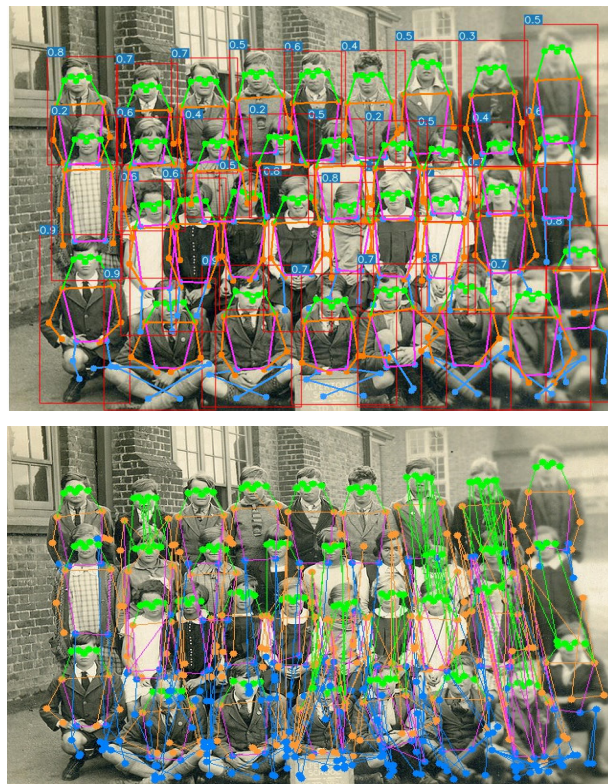
Figure 1. Qualitative result on a crowded COCO val2017 sample image. Top: Output from yolov5m6-pose shows the robustness of our approach. Keypoints of one person is never mistaken with another because of inherent grouping. Bottom: Output from HigherHRNetW32 showing how easily the grouping algorithm fails even when the keypoint locations are mostly correct. Bottom-up approaches are prone to such grouping errors in crowded scenes.
