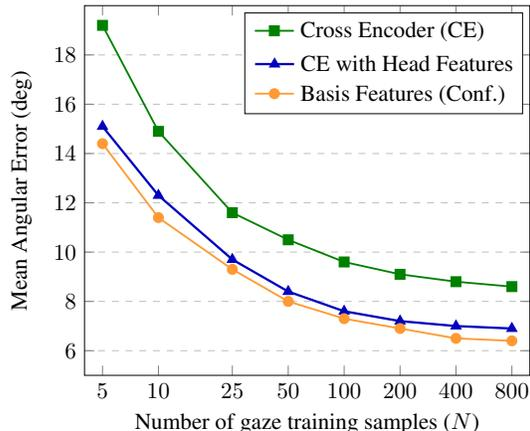
Figure 4. **Gaze estimation performance under  $N$ -shot training.** The addition of head features and multi-view self-supervision to cross-encoder training uniformly improves few-shot gaze estimation performance by a significant margin (20% on average), while using confidence-weighted basis features improves performance still further (24% on average).
