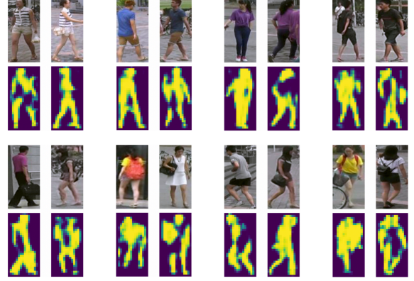
Figure 11. Sample segmentation and matching results on Market-1501 dataset. On the first 2 rows we illustrate matching and figure-ground segmentation masks and on the third and fourth rows non-matching pairs. The segmentations are obtained with using SCOTT which was trained on Human3.6M only.
