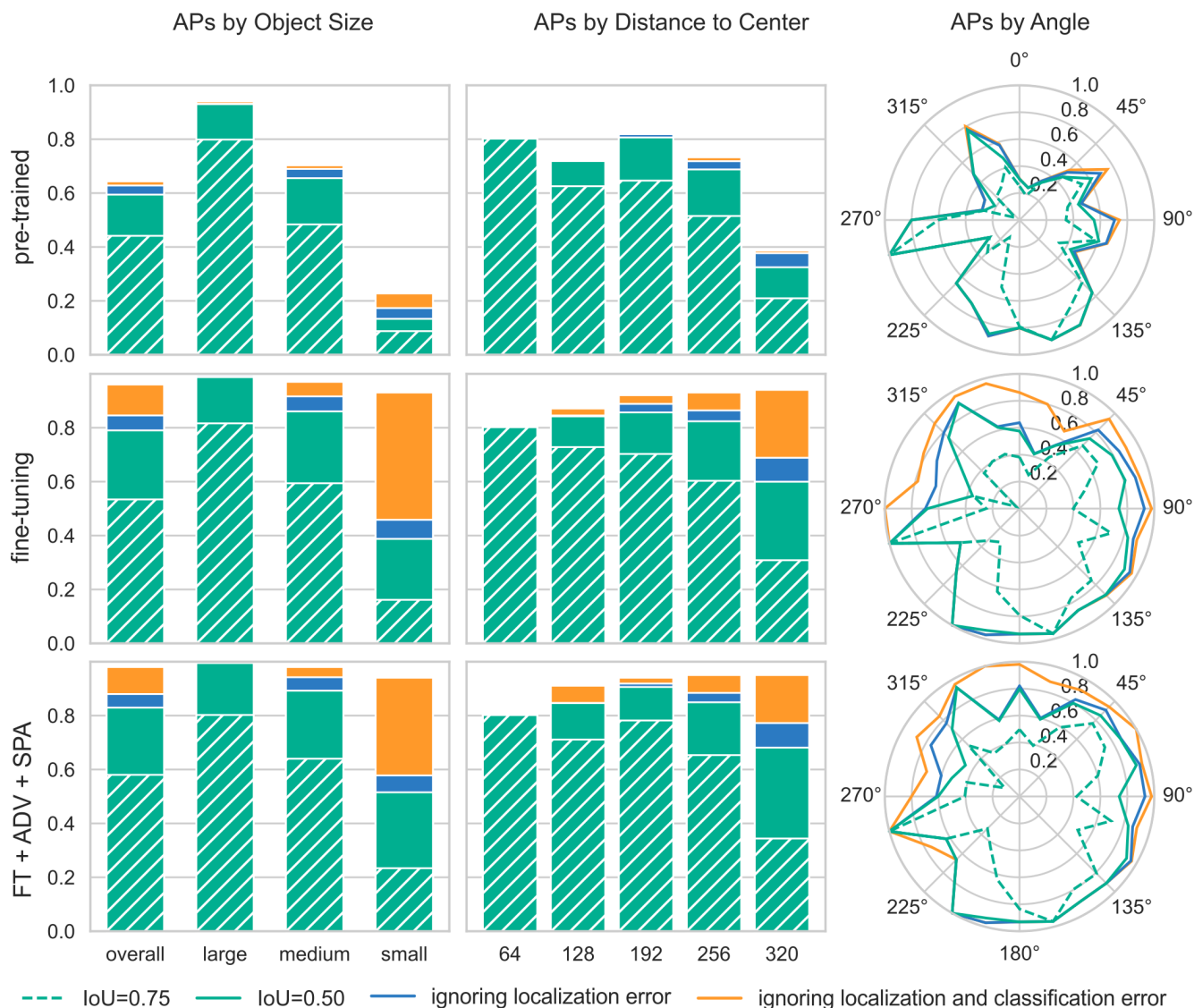
Figure 4. Model performance measured as AP across object size (left), distance to image center (center), and angle of rotation (right) on PIROPO for the pre-trained model without fine-tuning (top), the fine-tuning baseline (middle), and the final method (bottom). Shown are the AP@75 (dashed/cross-hatched green), AP@50 (green), AP@10 (blue), and AP@10 with corrected classifications (orange). AP@10 corresponds to the model’s performance if all bounding boxes were predicted correctly, and AP@10 with corrected classifications corresponds to performance if all detections had been correct. The difference between this last metric and 100% is due to objects left entirely undetected.
