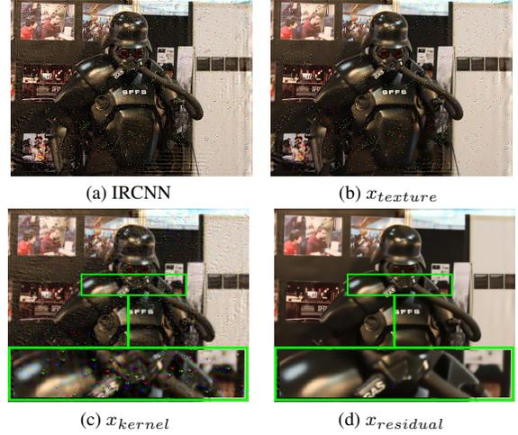
Figure 4. The deblurred results of (a) IRCNN (b) the proposed method only considering the texture reserving prior (c) the proposed model only considering only the kernel error term and (d) the proposed model considering only the residual error term.
