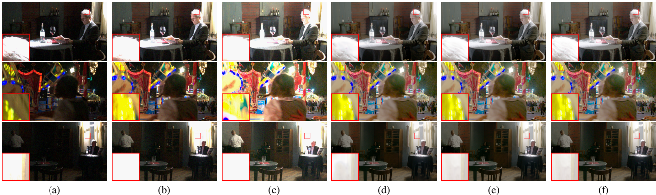
Figure 7. Qualitative comparison of our EAPNet with SOTA method AHDR. Fig. 7a, Fig. 7b and Fig. 7c are short, medium, and long exposed LDRs respectively. The HDR images restored by AHDR are shown in Fig. 7d, and the HDR images restored by our standard EAPNet are shown in Fig. 7e, and the HDR ground-truth images are shown in Fig. 7f.
