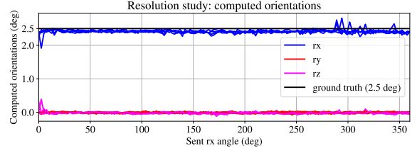
Figure 3. Accuracy test carried over the whole images data-set, with a ground truth of 2.5 deg between successive images.
