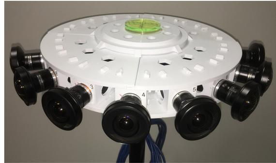
Figure 1. Our 360° camera array comprising 16 fisheye cameras
