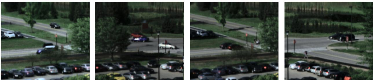
(c) Vehicles occluded by other vehicles in the scene. The second figure from the left also shows the image perturbations caused by glint in the scene.
