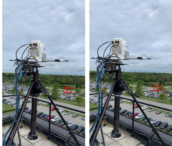
(a) Data acquisition with the Headwall Hyperspec. We focus on a red vehicle of interest to show the details captured via spectral imagery.
