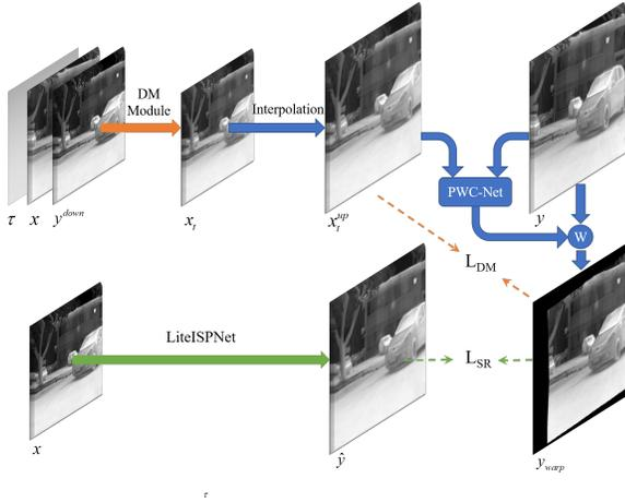
Figure 7: Architecture proposed by NPU-LIFT-LAB.
