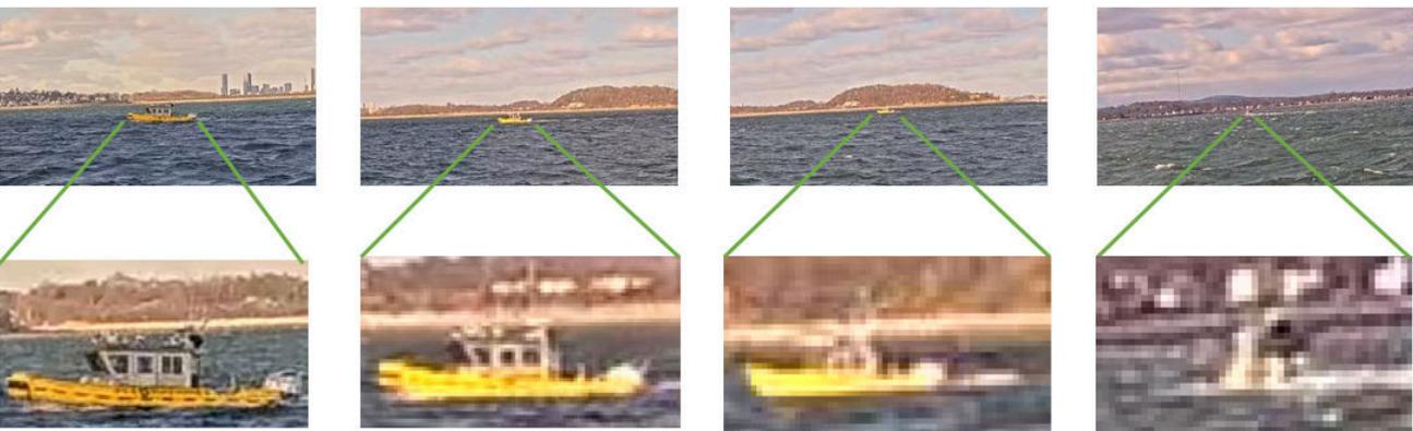
(f) Scale variability. The scale of objects decreases as the distance increases. Vessel size in pixels [Left to right]: 140×40, 75×20, 38×12, 12×11. Smaller objects that are only a few pixels in size can be hard to detect, classify and track.
