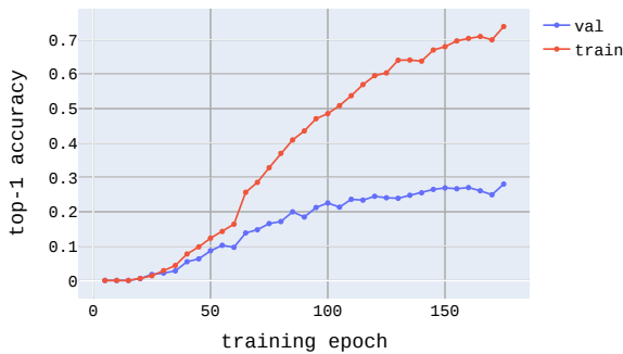
Figure 4. Generalization gap of curriculum adversarial training – The generalization gap keeps increasing as the curriculum training proceeds. The x -axis is training iterations and the y -axis is the top-1 accuracy. The red and blue lines indicate the top-1 training and validation accuracy, respectively.
