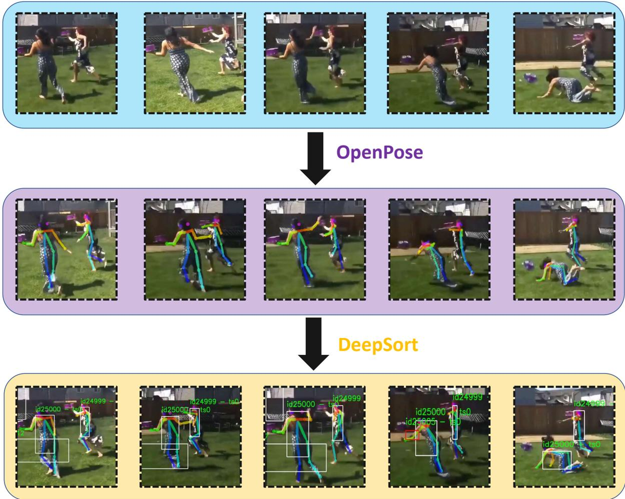
Figure 3. An example of extracting body keypoint coordinates of multiple agents in videos using Openpose [1], followed by Deepsort [18] to cluster the keypoints of the same person across the frames.
