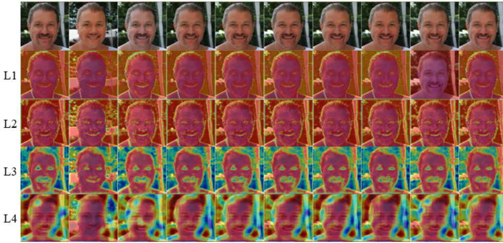
Figure 5. Attention maps of the first four layers (L1, L2, L3, L4) of the Resnet-18 trained for the a-priori known model classification task.
