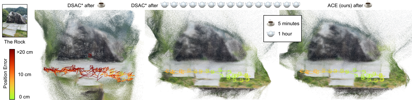
Figure 5. Qualitative results. We compare qualitative results of ACE and DSAC* on one scene of the Wayspots dataset. Full training of DSAC* takes 15 hours. When stopped after 5 minutes, relocalization accuracy is poor. We show the learned map for each method.
