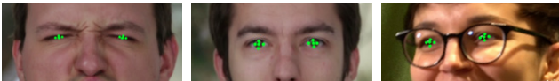
Figure 12. Our method can predict high quality eye landmarks, which could be used in eye tracking applications.
