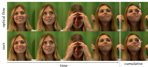
Figure 7. Our method allows to track user-defined features across a video, as shown by the pink dot on the eyebrow. In contrast to optical flow tracking [2], our method is not affected when the face point is occluded.
